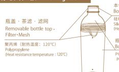
本体密封件・瓶盖密封件 Bottle gasket • Cap gasket 硅橡胶 (耐热温度: 180°C) Silicone rubber (Heat resistance temperature : 180°C)
