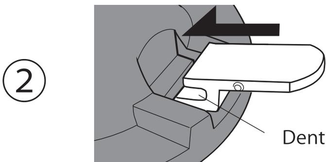
Flip it over and set the switch onto the base as shown in the diagram. Confirm that the switch moves up and down before use.
