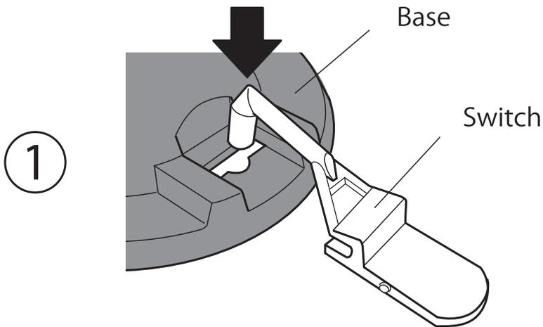
Stick the long narrow end into the hole of the base. Then insert it all the way in up to the base of the switch.
